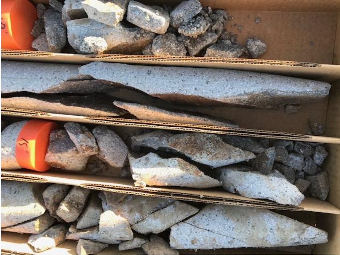
Photo 7 – Core “loss” at 0 – 8 feet. Why was core not collected from the surface to 8 feet?
