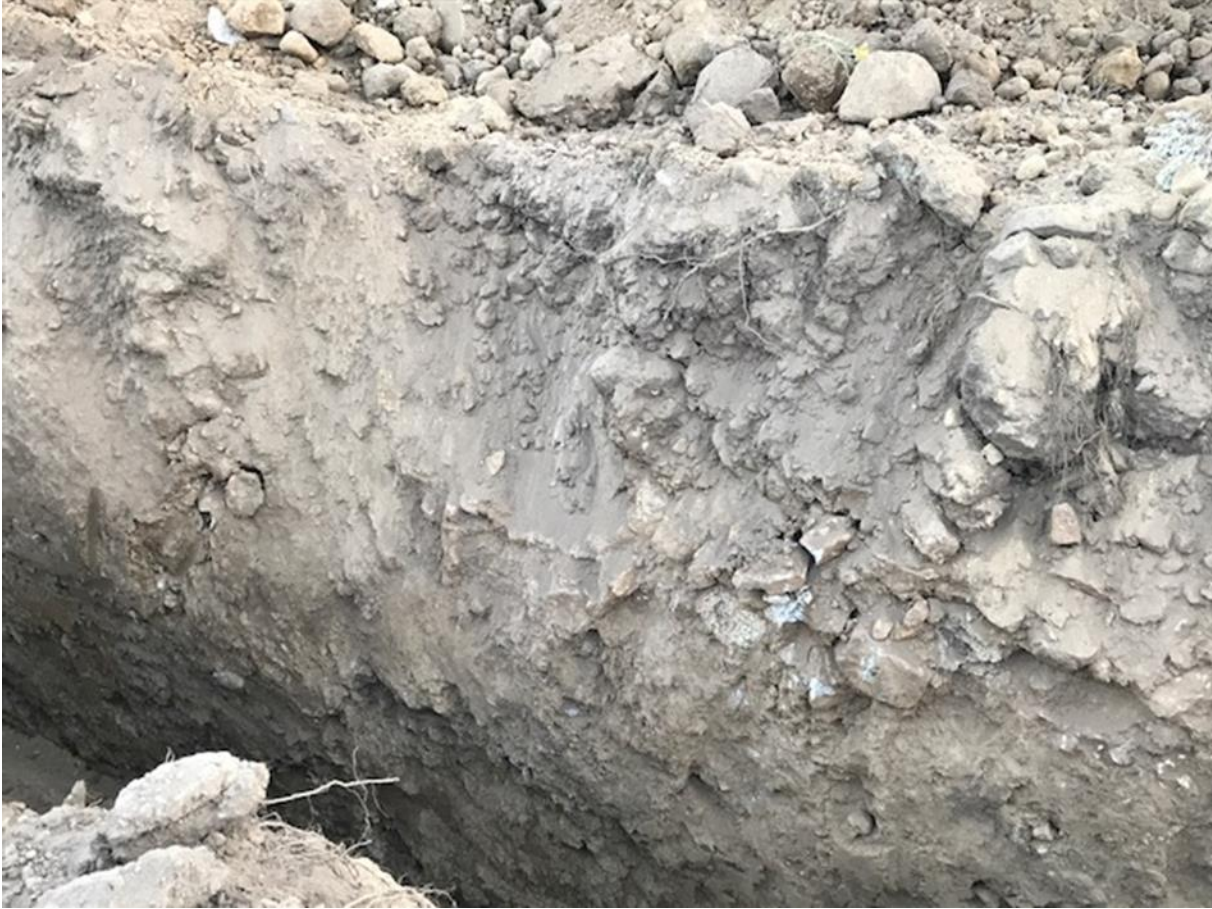
Photo 3 - Fault trace in trench just south of Brushwood Way on west side of Ascenté property. If the trench walls had been scraped smooth, the changes in the rock facies would have been more apparent.
