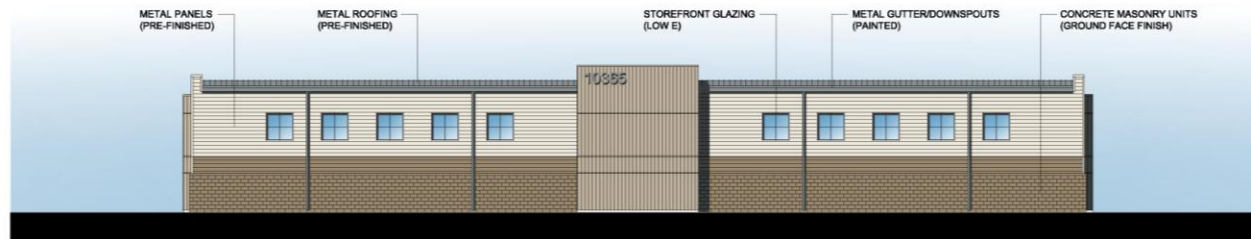
North Elevation (I-80)
