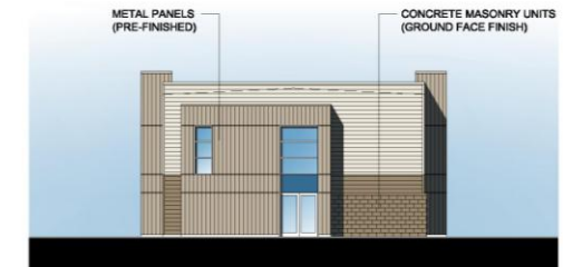
East Elevation (Interior)
