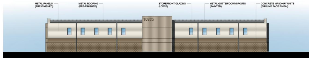
North Elevation (I-80)
